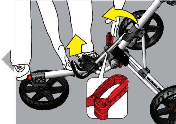
**5** Still stepping on the front wheel, pull up on the lower bag support and lock the main hinge LEVER.
