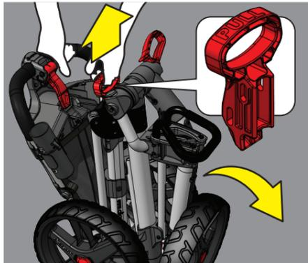
**2** Pull the LATCH and lower the cart onto the front wheel.
