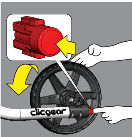
**1** Push the front wheel BUTTON and rotate the front wheel to the horizontal position.
