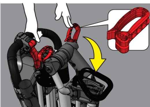
**6** Lift the cart onto its wheels and lock the main hinge LEVER.
