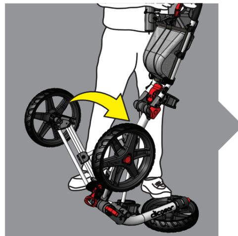
**3** With your foot on the front wheel, fold the handle back towards the front wheel.
