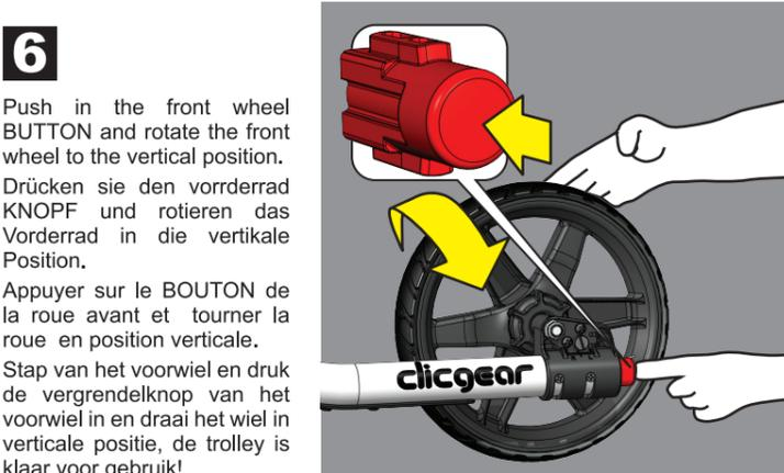
**6** Push in the front wheel BUTTON and rotate the front wheel to the vertical position.
