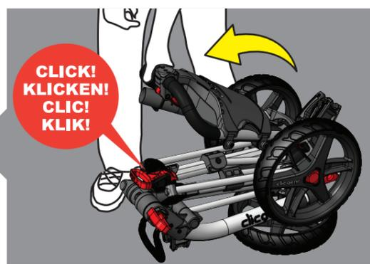
**5** Push the handle down onto the cart until it CLICKS and locks the handle in place.
